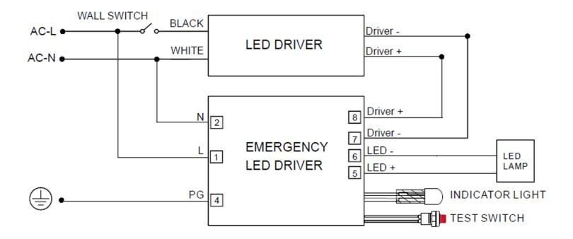
Wiring diagram for applications where the LED fixtures output is MORE than 120w and the fixture LED Driver Current output is NOT to exceed 6A.
